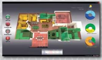
All energy and water usage information is displayed in the house on a touch-screen interface, that can be accessed remotely via the internet or a mobile phone. The display will show the occupants at-a-glance energy consumption of different appliances in the house (e.g. the air conditioner) or of specific zones (e.g. living areas or kitchen).
