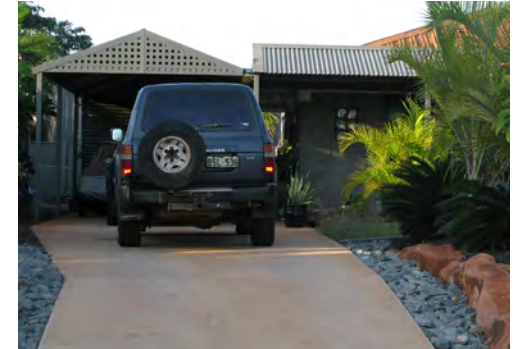
Use of local stone for landscaping and loose stone along the edge of the driveway are effective ways to provide good on-site drainage especially on a sloping site - Dampier
