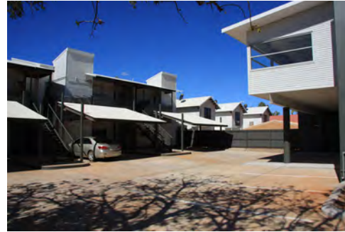
For cyclone management separate carport roof from main roof - Broome
